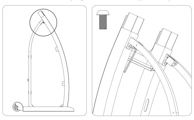
STEP 5: Secure the side panels to frame using  $12 \times 68$  screws - A Phillips screw driver is required for this step. Repeat for opposite side.
