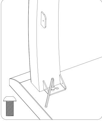
STEP 4: Secure the rear arms to front assembly using 2 x M8 x 16mm screws and supplied M8 Hex Key.
