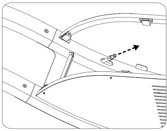
STEP 10: Secure the heater head to arms using 4 x M8 screws and supplied washers with M8 Hex Key.
