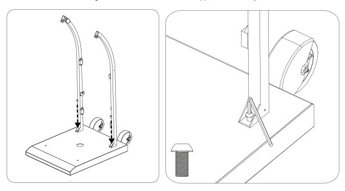
STEP 3: Position front assembly and fasten using 2 x M8 20mm screws using supplied M8 Hex Key.
