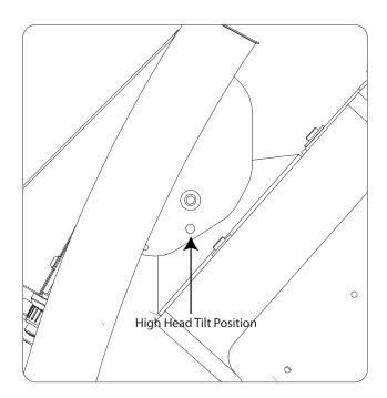
To set heater head angle at high position, manually push heater head up to align hole then insert slip pin.
