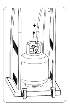
STEP 17: Lower gas bottle bracket into position.
