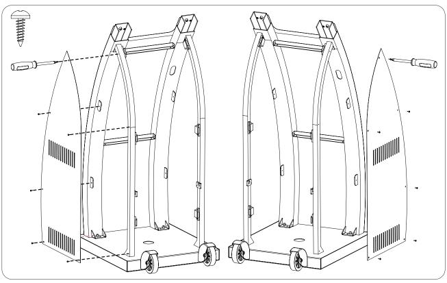
STEP 6: Slide top arms over front assembly slip joints - Ensure top screw holes are faced inwards. Secure the front panel to top arms using  $4 \times M5$  screws.
