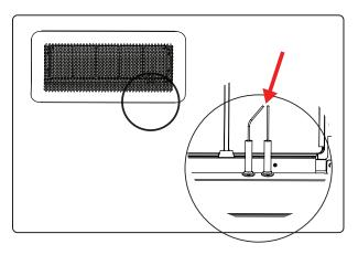
5. Once at IGNITION position, press control knob while simultaneously pressing the spark ignition button. Continue to hold in controls for 10 seconds for ignition to complete.
