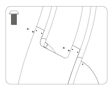
\* Note: The joint between the lower and upper arms is firm to ensure` rigidily and stability of the product. To engage slowly lever the two sections together using some force and push down fully
