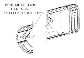
Hold the new emitter by the ceramic ends or wear clean dry gloves to prevent and position the new lamp inside the unit.
