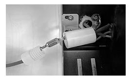
10. Carefully replace the protective aluminum grille and screw the protective end cap in place.
