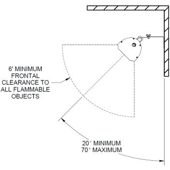
The angles of attachment are 20° to 70°, measured from the mounting wall.
