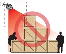
Failure to observe stated clearances to combustibles will result in a fire hazard. Failure to properly denote hazard may also result in a future hazard.
