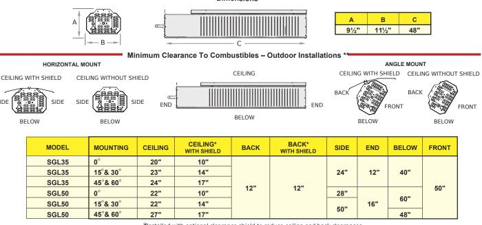
\*Installed with optional clearance shield to reduce ceiling and back clearances.
