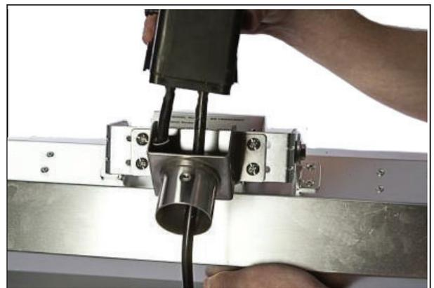
**4** Align Tilt Switch (black box on **Head Unit 1**) to threaded holes on **Mounting Bracket 2**, then secure with small screws and flat washers.
