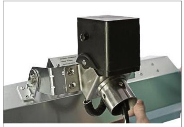
**5** Thread electrical cord through **Curved Upper Arm 3** and attach with 4 threaded bolts and lock washers. Ensure that tilt switch (black box) stays horizontal/level.
