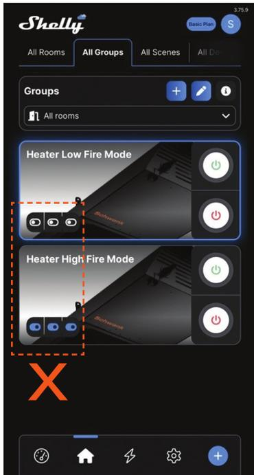
If the high fire mode is ON while turning OFF low fire mode, the heaters will be turned off, even though high fire mode is shown "ON" from the app.
